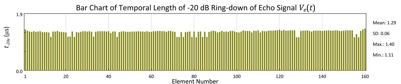
Note:  $t_{r20e}$  would be more sensitive to system noises especially in the situation of low SNR
