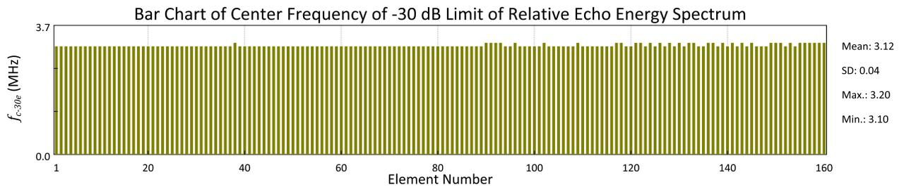
Note:  $f_{c-30e}$  would be more sensitive to system noises especially in the situation of low SNR
