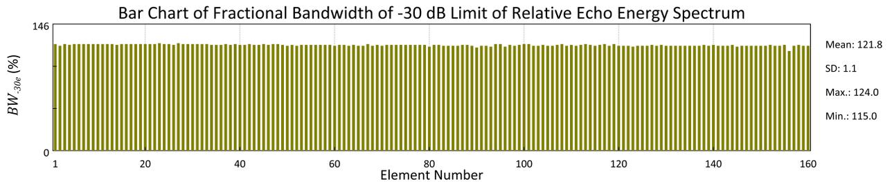
Note:  $BW_{-30e}$  would be more sensitive to system noises especially in the situation of low SNR
