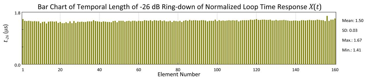
Note:  $t_{26}$  would be more sensitive to system noises especially in the situation of low SNR
