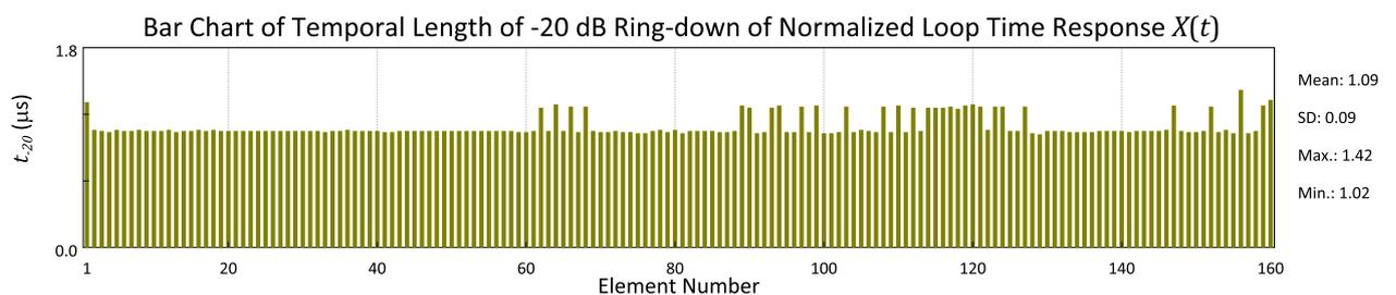
Note:  $t_{20}$  would be more sensitive to system noises especially in the situation of low SNR
